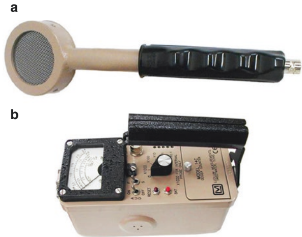
Fig. 3.3 A Geiger–Müller survey meter. (a) Ludlum pancake probe model 44-9. (b) Ludlum model 14C survey meter (Photo courtesy of Ludlum Measurements, Inc.)
